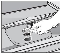
■ Replace the combination filter so that it lies flat in the base of the wash cabinet. Secure it by turning the handle clockwise.
